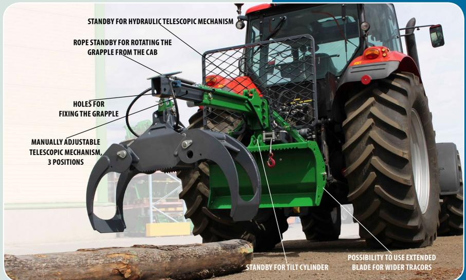
Grapple skidder is available with manual pull-out or hydraulic telescopic mechanism. Operations are possible with the tractor's hydraulics. As an extra option to the grapple skidder, we offer the FARMA winch RW600S that can be controlled via the tractor or via radio control.
